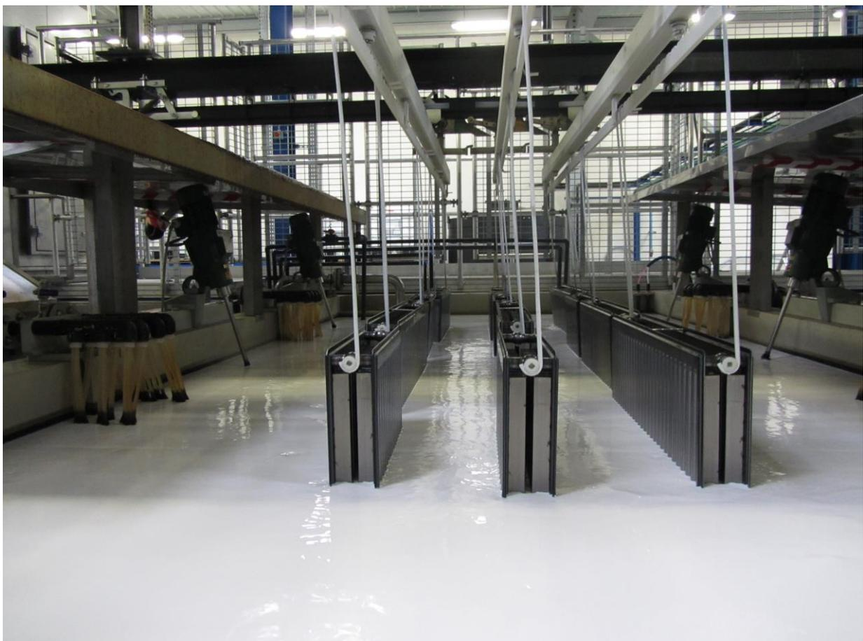
Radiators being immersed in the BONDERITE M-PP 102 tank.
