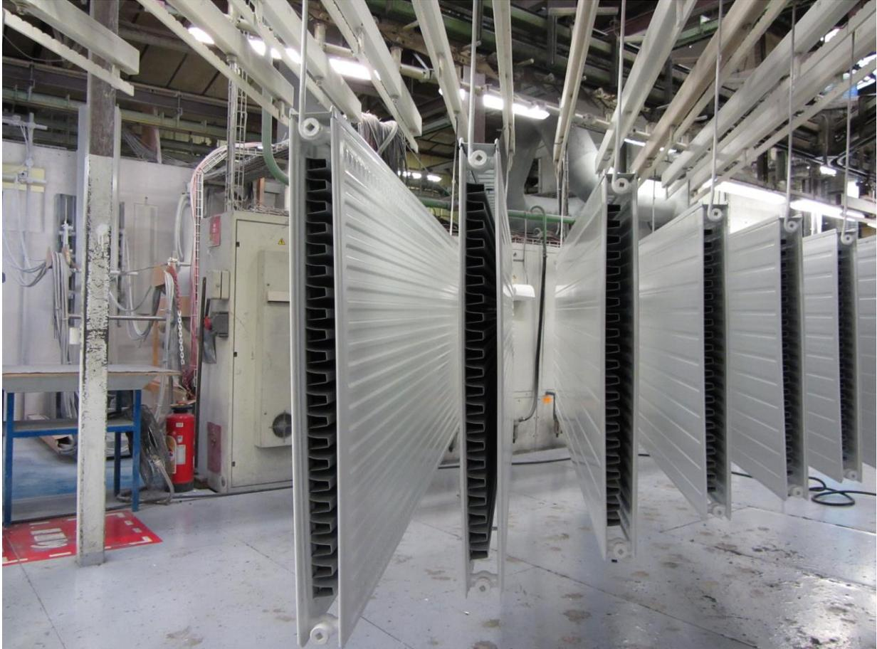
Radiators having just exited the co-curing BONDERITE M-PP 102 + powder paint oven.
